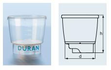
Designed for sterilization or clarification of aqueous cell culture media Supplied as a filter funnel unit for use with the DURAN<sup>\*</sup> *TILT* bottle (with GL 45 thread adaptor) or 45 mm media bottles. Comes in three different asymmetric pore sizes (0.1  $\mu$ m, 0.2  $\mu$ m, or 0.45  $\mu$ m). Raised moulded graduation marks for easy volume reading. Manufactured in a Class 100,000 clean room from Class VI, non-cytotoxic materials. Supplied sterile.
