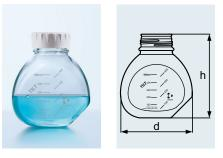
The DURAN<sup>\*</sup> *TILT* bottle has two positions: upright for filter sterilization or storage, and tilted at 45° for pipetting. The bottle systems allows working with cell culture media under sterile conditions in biosafety cabinets and clean hoods.
