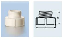
The re-usable adaptor (GL 45 external / GL 56 internal) allows the use of the DURAN<sup>®</sup> *TILT* bottle with 45 mm filtation units for the filter sterilisation of cell culture media. Manufactured from inert PTFE; can be autoclaved and depyrogenised at 300 °C.
